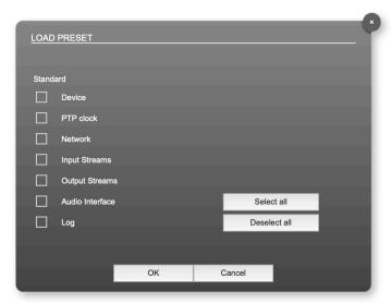
The device configuration can be stored to a single file (.rps). Restoring the configuration a dialog prompts for selection of individual settings.
