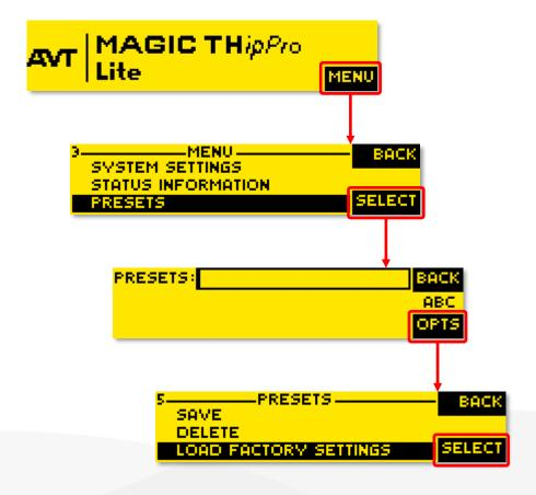
If there is a password configured but the password is not known, the device can only be reset via front display as shown on the right.
