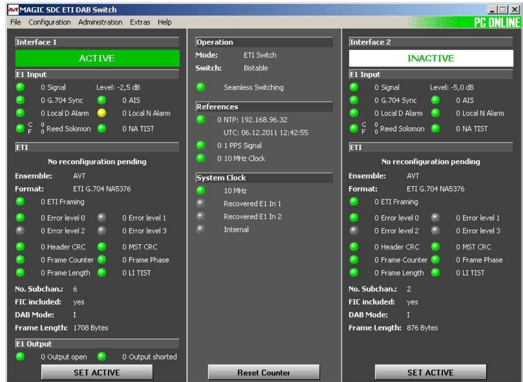
FIG. 3 MAIN WINDOW - ETI SWITCH
