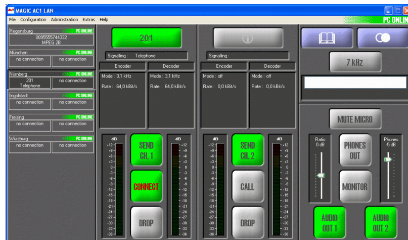
FIG. 84 MAIN WINDOW: CONTROL OF SEVERAL AUDIO CODECS
