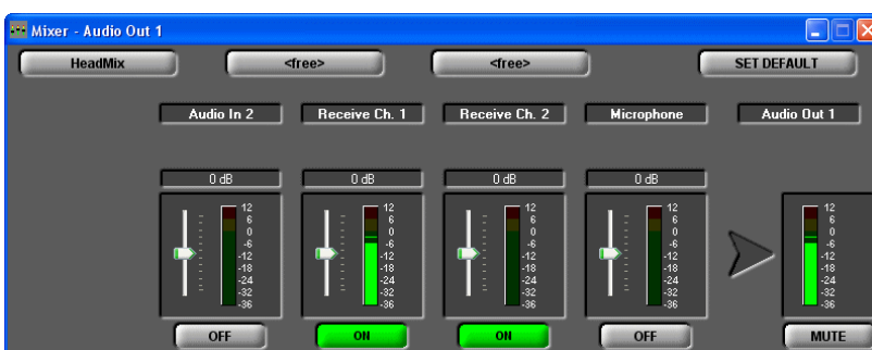
FIG. 15 AUDIO MIXER AUDIO OUTPUT
