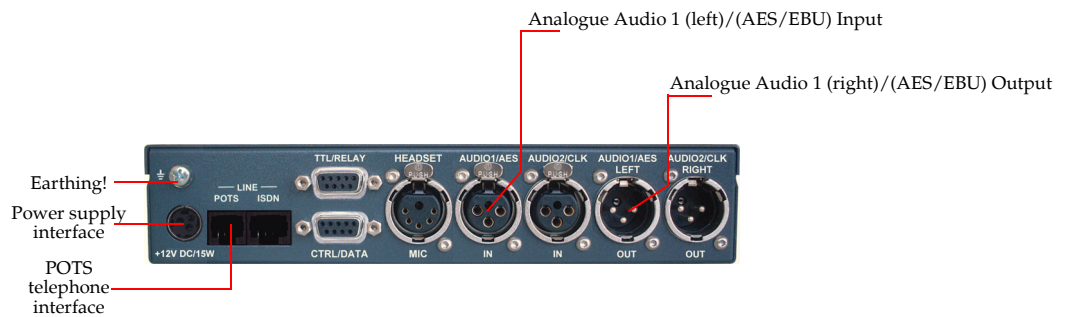
FIG. 5 MINIMUM WIRING FOR ANALOGUE POTS OPERATION
