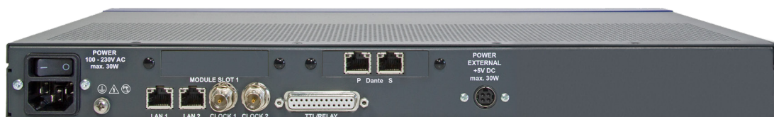
MAGIC THipPro Pure Lite with Dante Module, redundant power supply (without conventional audio interfaces)
