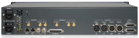
MAGIC TBR equipped with two RF modules – Rear side
