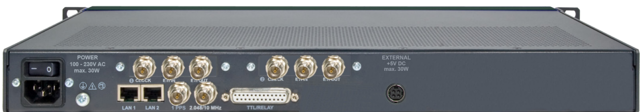
MAGIC SDC with 2 x ETI modul and redundant PSU – Rear side
