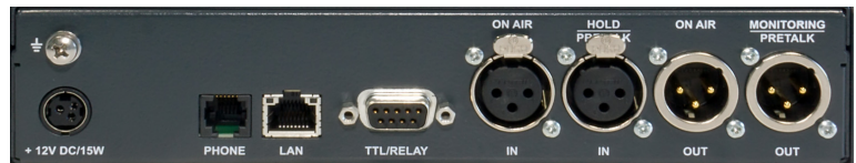
FIG. 10 REAR VIEW OF THE MAGIC TH1IPGO TELEPHONE HYBRIDS
